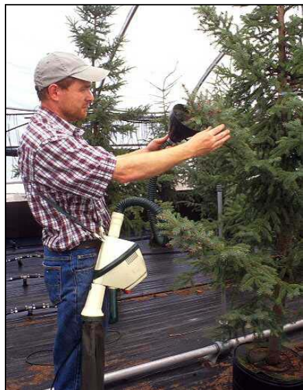
Figure 3. Vacuum apparatus used to collect pollen. Pollen is collected the same day it is disseminated, thus ensuring its quality. (Photo: S. Mercier, MRNFP)
