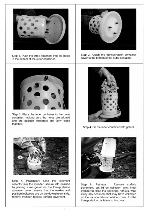
FIGURE 2.—Six steps for the use of the SÉDIBAC 45 sediment collector, from mounting to retrieval.
