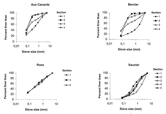
FIGURE 3.—Grading curves of fine sediment (diameter < 5 mm) accumulated in the SÉDIBAC 45 in the first autumn (2000) following culvert construction, for each study section of the Aux Canards, Bernier, Roza, and Saunier streams on the Laurentian Shield, Québec.
